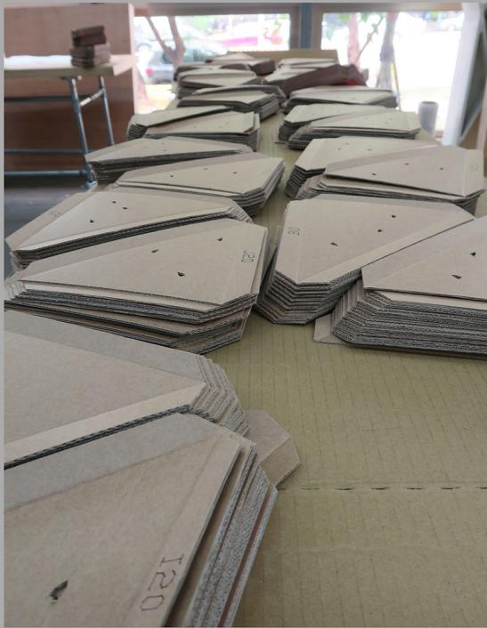
The most challenging point of constructing Spiral Pavilion is the accuracy of a digital file, and by hand construction. Each part of the pavilion is labeled by CNC machine, which can also cut and press for folding lines. Since cardboard material is not necessarily rigid material to create enough structural strength, the design for parts joint and details needed to pay a lot of attention.
